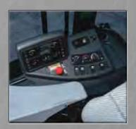
Diagnostics have been made simple with the state-of-the-art multi-function display panel which provides at-a-glance information via 16 warning lights, 5 gauges and dual function LCD.
