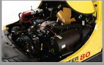
The engine cover, hinged at the rear, offers superior service access to the engine compartment with an opening angle of 85 degrees. The tough engine cover is made of a durable, crack-resistant, thermoset polyester resin reinforced with fiberglass.
