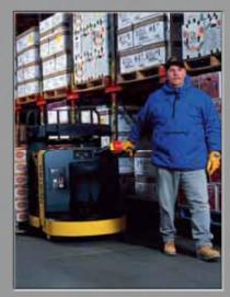
In cold room and freezer applications, your pallet trucks require protection. That's why Hyster offers two optional application/ environmental packages for low temperature applications; the cooler/freezer package for temperatures from 0°F to 120°F and the SubZero Freezer Package for temperatures from -40° to +120°F.
